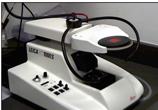
Above: Leica Vibratome; Above right: Nikon microscope set-up
