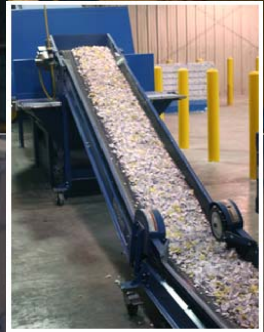
Additional conveyors feed our fully automated high production baling system.
