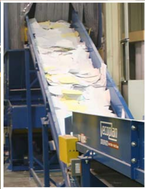
Confidential documents are conveyor fed to the shredder.
